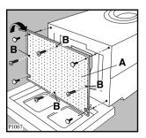
6. Set the machine upright and remove the two remaining bolts from the back.
